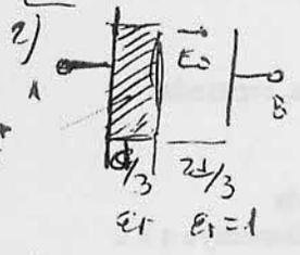
$V = E_0 \frac{2d}{3} + E \frac{d}{3} = E_0 \frac{2d}{3} + \frac{E_0}{\epsilon_r} \frac{d}{3} = E_0 \frac{d}{3} \left( 2 + \frac{1}{\epsilon_r} \right) = \frac{V_0}{3} \left( 2 + \frac{1}{\epsilon_r} \right)$
