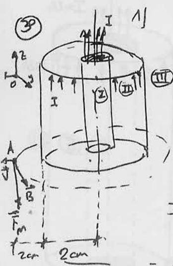
$$\oint \vec{B} \cdot d\vec{l} = \mu_0 I_c = \oint B_{\phi} dl = B_{\phi} \cdot 2\pi r = \mu_0 \frac{4r^2}{d^2} I \Rightarrow B_{\phi} = \frac{2\mu_0 I}{\pi d^2} (r)$$
