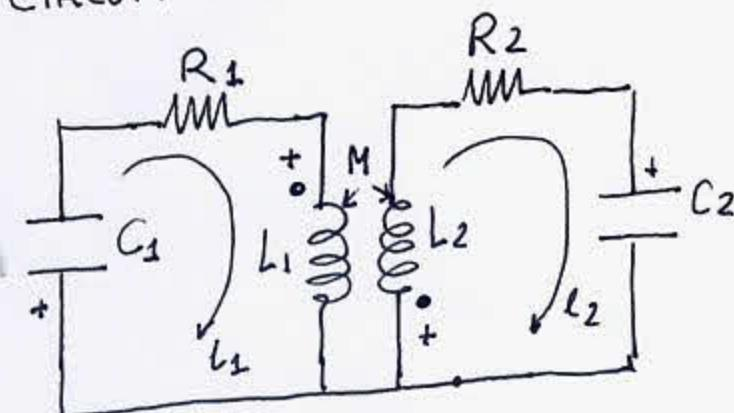
$$L_1 \frac{di_1}{dt} + M \frac{di_2}{dt} + l_1 R_1 + \frac{1}{C_1} \int_{0}^{t} i_1 dt \pm \frac{q_1(0)}{C_1} = 0$$
