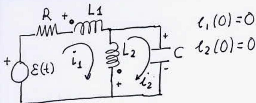
$$l_1 R + L_1 \frac{dl_1}{dt} + M \frac{d(l_2 - l_1)}{dt} + L_2 \frac{d(l_1 - l_2)}{dt} + M \frac{dl_1}{dt} = E(t)$$
