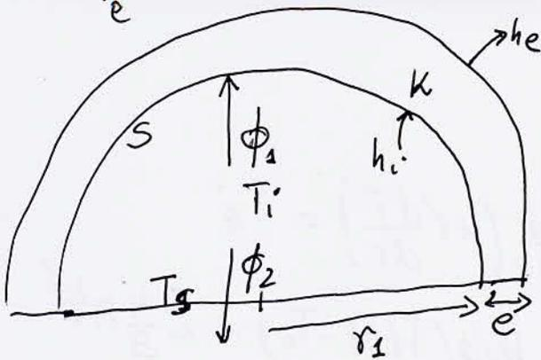
$$\phi_T = \phi_1 + \phi_2 = \frac{T_i - T_e}{\frac{1}{h_i \cdot S_i} + \frac{1}{2\pi k} \left( \frac{1}{r_1} - \frac{1}{r_2} \right) + \frac{1}{h_e S_e}} + h_i \cdot S_s \cdot (T_i - T_s)$$
