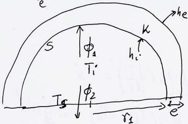
$$\phi_T = \phi_1 + \phi_2 = \frac{T_i - T_e}{\frac{1}{h_i \cdot S_i} + \frac{1}{2\pi k} \left( \frac{1}{r_1} - \frac{1}{r_2} \right) + \frac{1}{h_e S_e}} + h_i \cdot S_i \cdot (T_i - T_s)$$
