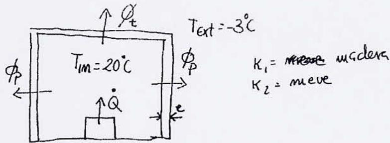
$$\phi = \phi_t + \phi_p = \frac{T_{im} - T_{ext}}{R_t} + \frac{T_{im} - T_{ext}}{R_p} = \dot{Q} = c \cdot M$$
