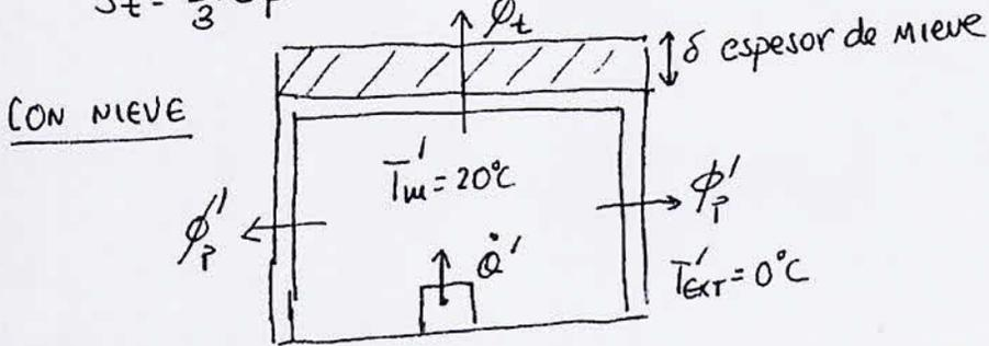
$$\phi' = \phi'_t + \phi'_p = \frac{T'_{im} - T'_{ext}}{R'_t} + \frac{T'_{im} - T'_{ext}}{R'_p} = \dot{Q}' = c \cdot M'$$
