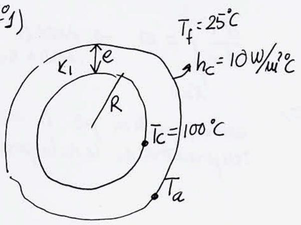
a)  $R_c = \frac{k_1}{h_c} = \frac{0,5}{10} = 0,05 \text{ m} = 50 \text{ mm}$
