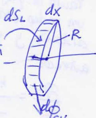
$$\begin{aligned} \phi_{cv} &= \int_0^\infty h\pi D dx (T(x) - T_\infty) = \\ &= \pi Dh (T_0 - T_\infty) \int_0^\infty e^{-mx} dx = \frac{\pi Dh (T_0 - T_\infty)}{m} = \underline{\underline{8,3 \text{ W}}} \end{aligned}$$
